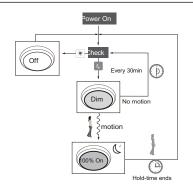
Difference between Corridor Function and Smart Photocell Function.
